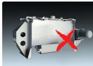
Ribbon mixer Bad mixing uniformity 65% loading rate
